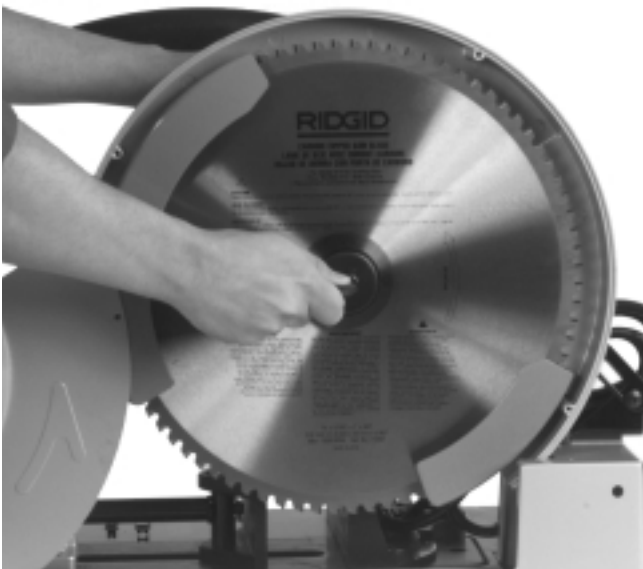
Figure 9 – Installing Saw Blade
